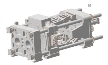
The central axle of rotary tale is coupled with two Japanese bearings which guarantees the best tolerance, solidness, quality and durability.
