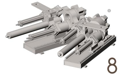
To shorten the pitch and the distance of two injection units, we develop this latest vertical two-cylinder structure for injection units.
